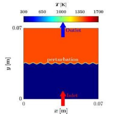
Numerical setup for the flame <sup>(Wen et al., 2023)</sup>
